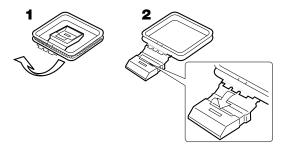
Place the antenna on a shelf, for example, or hang it on a window frame, etc., in the direction which gives the best reception, as far away as possible from the entire system, speaker cords and the power cord to prevent unwanted noise.
